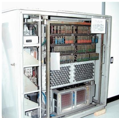
図-5 ETL Mark IV A
